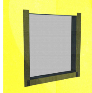
Extend AquaFlash System to interior of wall.
